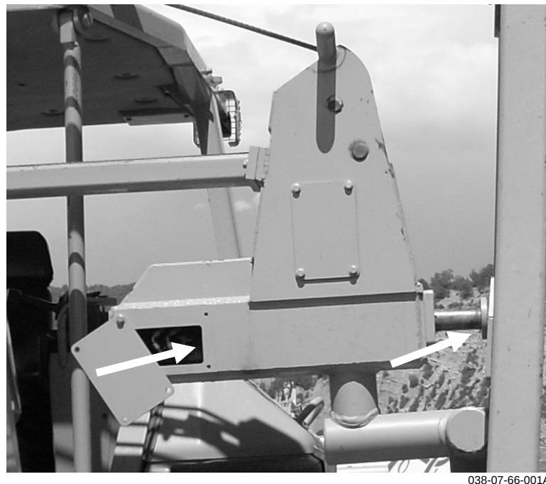
Figure 43: Check inner and outer boom stop bushings.
